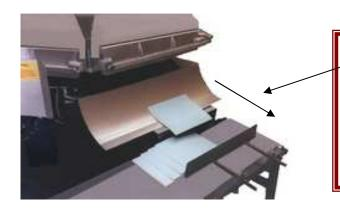
The angle of the conveyor bed matches the precise angle of the **Circular Padder** delivery chute, allowing pads to slip smoothly on to the belt, either in a constant, shingled stream or stacked against the workstop. The speed of the belt can be adjusted up or down as desired.
